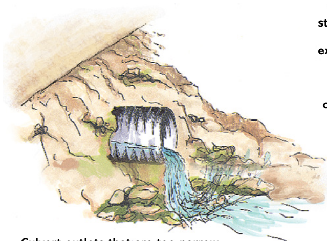
Culvert outlets that are too narrow and set too high cause water to undercut the road fill and streambed.
