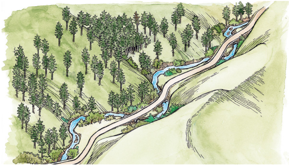
UNACCEPTABLE OPTION: Roads built or reconstructed next to a stream channel with multiple crossings are not allowed. Note: Many older roads and highways are in such locations.
