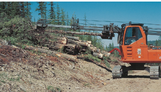
The stroke-boom de-limber operates at the landing or roadside, removing tree limbs and tops, cutting the stem into logs and stacking them.
