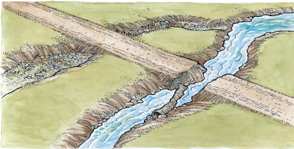
Early road construction techniques often filled side channels and contributed to the failure of main channel culverts during high-water events.
