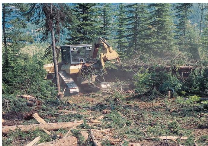
This crawler tractor, equipped with a grapple, picks up whole trees and moves them to a landing or roadside.
