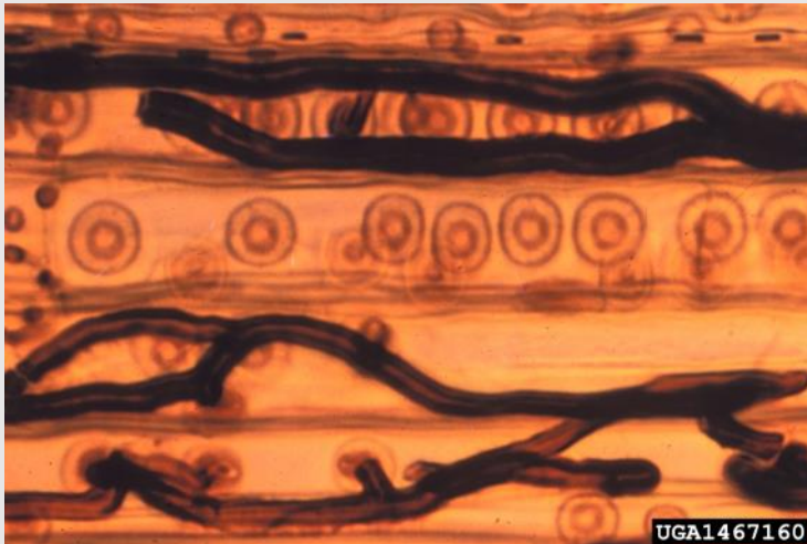
Fungal hyphae passing through pits of Douglas-fir tracheids.
